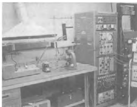
Figure 3-3. ABOVE: Kamentsky's Rapid Cell Spectrophotometer, as shown in several publications; this is actually the third version of the instrument. BELOW: The real first RCS prototype, warts and all (courtesy of L. Kamentsky).
